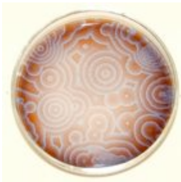
Patterns formed by chemical waves in the Belousov-Zhabotinsky reaction. Photo: Stephen Morris, University of Toronto.
