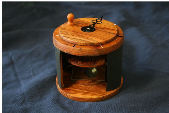
The Viking Sunstone Compass made by researchers at the University of Rennes. Note the double bright spots in the cavity.
