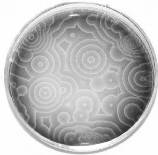
Figure 19 Chemical waves in the Belousov-Zhabotinsky reaction. Image: Stephen Morris, University of Toronto.
